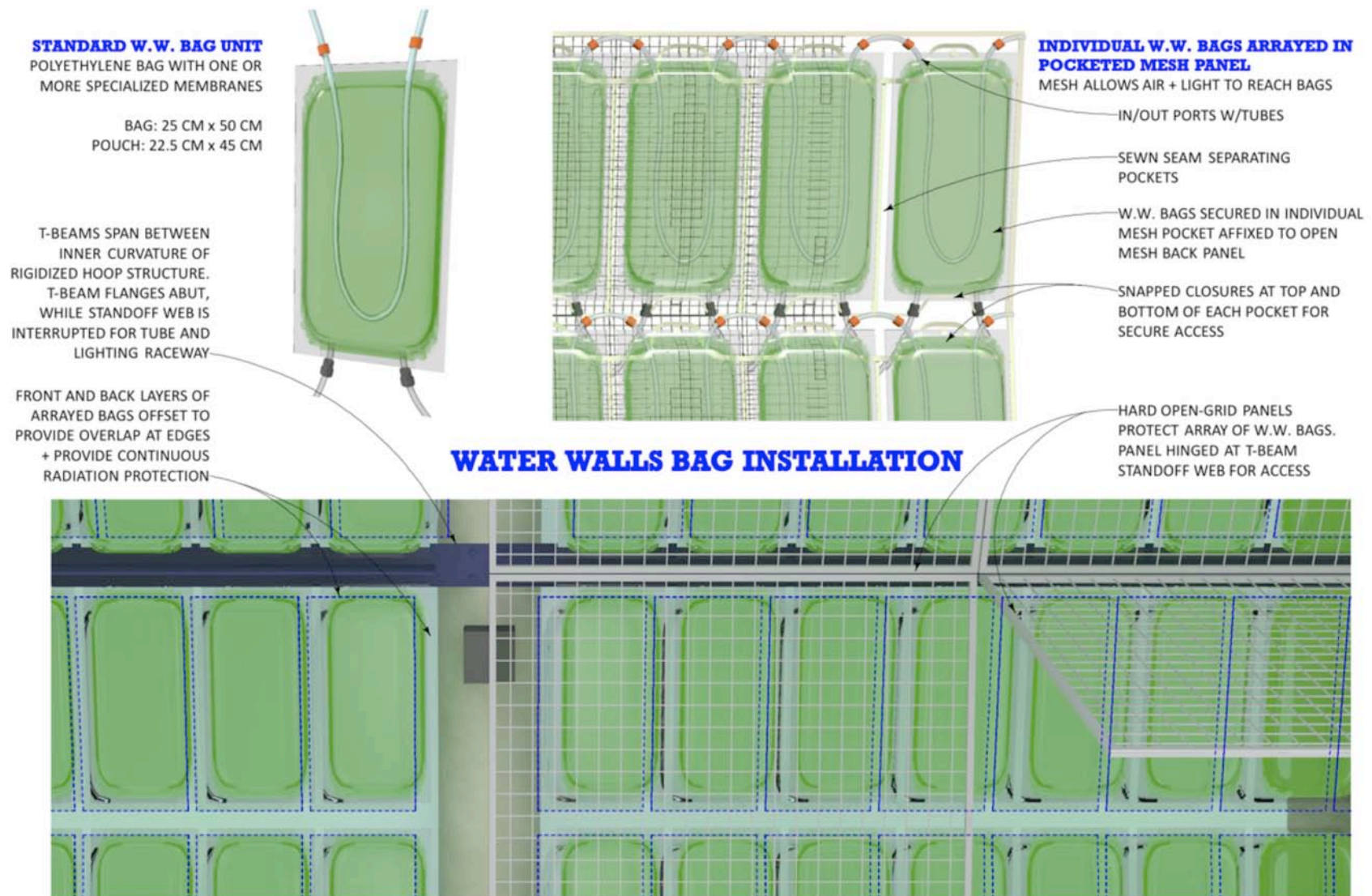
FIGURE 12. Installation of the Air Revitalization / Algae Growth Subsystem in a Habitable Space Module. Design Credit: Renée L. Matossian. Drawing Credit: François Lévy.
